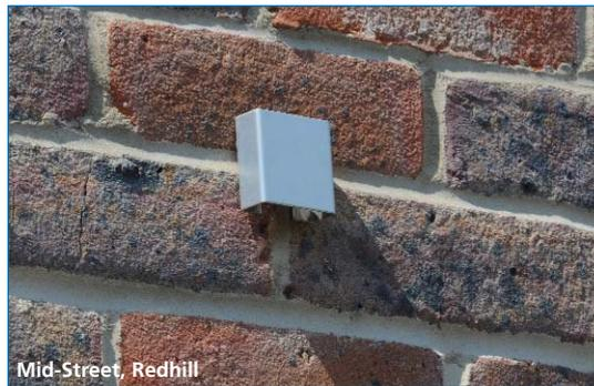
Figure 8: External temperature reader
